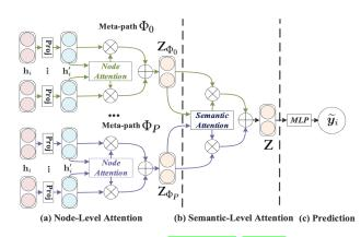
Fig. 16.5: The architecture of HAN (Wang et al, 2019m). The whole model can be divided into three parts: Node-Level Attention aims to learn the importance of neighbors' features. Semantic-Level Attention aims to learn the importance of different meta-paths. Prediction layer utilizes the labeled nodes to update node embeddings.
